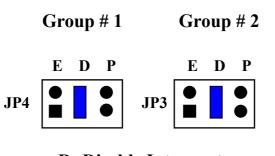
D: Disable Interrupt E: Enable Interrupt P: Programmable Interrupt
